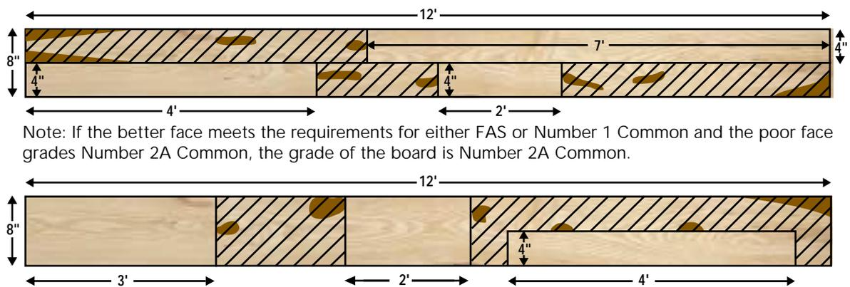
There are lower NHLA grades than Number 2A Common but they are usually converted into dimension parts, flooring parts, or used domestically in the USA.
